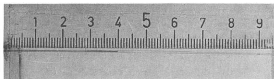
Fig. 3. Neutralization boundary created in the column revealed by addition of 0.0001 M phenol red to the primary electrolyte. Conditions: primary electrolyte, 0.01 M KCl; modifying electrolytes, 0.01 M KCl + 0.001 M HCl, 0.01 M KCl + 0.02 M ammonia solution; total current through column, 400 \mu\text{A} ; I_{\text{H}} = 50 \mu\text{A} ; I_{\text{OH}} = 100 \mu\text{A} . Photograph taken in 5 min.
